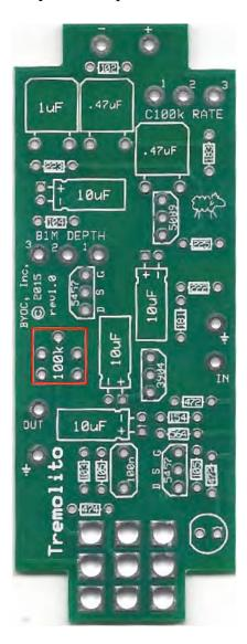
**Setting the Trimpot:** This is a simple output level trimpot. With the effect engaged, play through while turning the trimpot until you achieve 'unity' or in other words, until the level of the effect when on is the same as the level of the bypassed signal.
