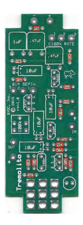
**Step 2**: Add the Trimpot. There are 5 holes in the PCB but only 3 leads on your trim pot. Don't let this confuse you. The extra holes are there to accommodate a variety of different brands/models. There should only be one way that your trimpot will fit into the PCB.
