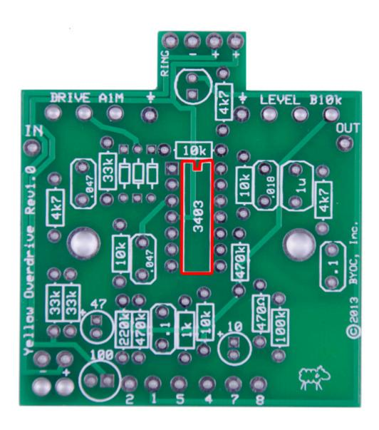
**Step 4:** Add the film capacitors. These are non-polarized so it can go in either direction.
