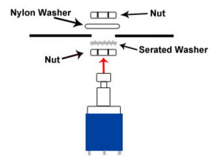
**Step 2:** Install the footswitch. Orient the footswitch so that the flat sides of the solder lugs are like the diagram below.
