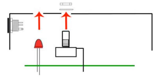
**Step 3:** Hold the PCB in one hand so that the component side of the PCB is in the palm of your hand and the bottom side with the pots, toggle switch and LED is facing up. Now use your other hand to guide the predrilled enclosure onto the PCB assembly so that the pots and LED all go into their respective holes. Once the PCB assembly is in place, secure it by screwing on the washers and nuts for the pots. Only tighten them with your fingers. You do not want them very tight yet.
