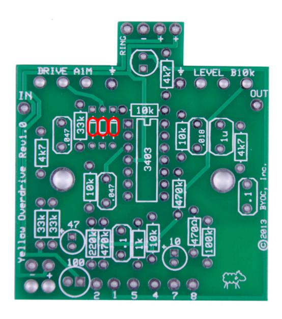
**Step 2:** Add all the resistors. Resistors are not polarized and can be inserted in either direction.
