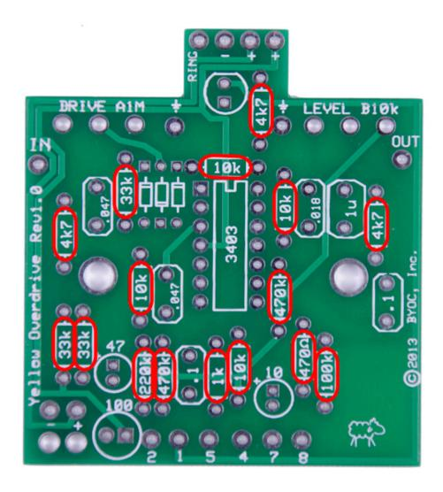
Step 3: Add the 14 pin IC socket. ONLY SOLDER THE SOCKET! NOT THE ACTUAL IC! This is a socket. The sockets get soldered to the PCB. The ICs get inserted into the sockets. The actual IC chip itself, never gets soldered. You will insert the IC into the socket after the entire pedal has been built.
